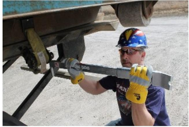
Throw away your winch bar. The T Handle, or Pistol Grip part of the Boom Dog Bar puts you in a comfortable position allowing you to easily tighten your nylon ratchet to the CORRECT spot.
