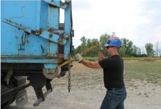
Container doors are heavy. No matter how well a container is built, they bend, and doors sag. Doors can be very difficult to close once they start to sag. The Boom Dog Bar lifts up saggy doors putting them back into a closed position.
