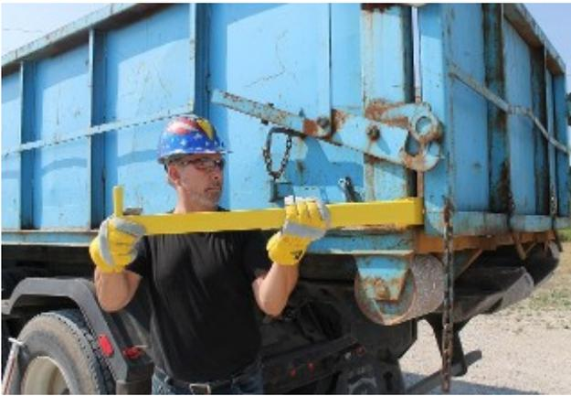
The most important feature of the bar, the prying feature. If the door does not release, drivers normally pull on the chain, or pushes open by hand, exposing arm and body to everything in the box. The prying feature will keep you safe at a distance.
