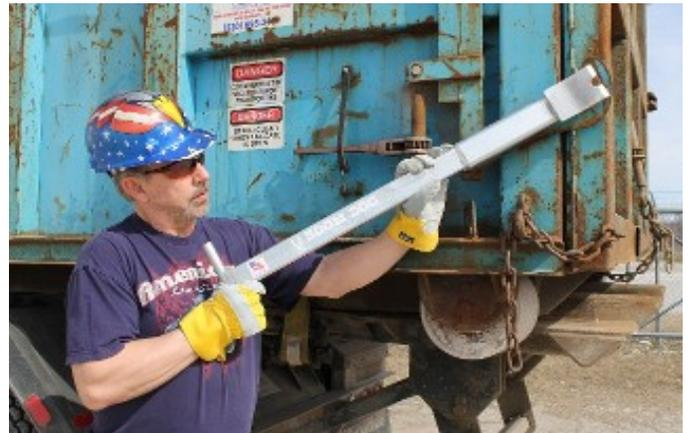
If the door still does not open the bar is designed with an opening to fit the door. The patented punch will kick open the door without ever having to expose your body.
